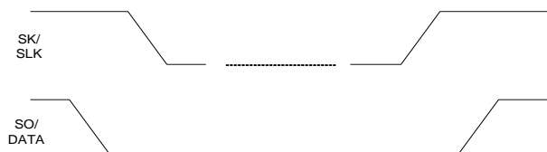
Figure 35: Timing of 2-wire START and STOP condition
