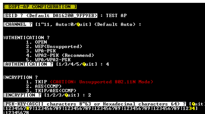
Figure 12: Set Up AP
