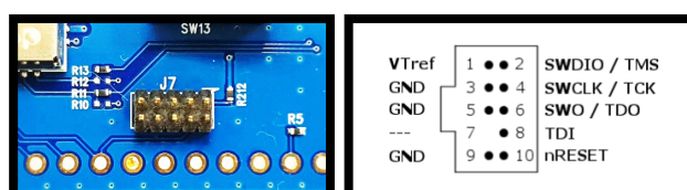
Figure 2: JTAG Pin Connection
