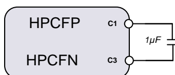
Figure 41: Charge Pump Flying Capacitor
