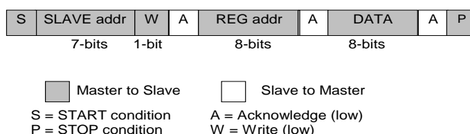
Figure 27: I 2 C Byte Write (SDA signal)
