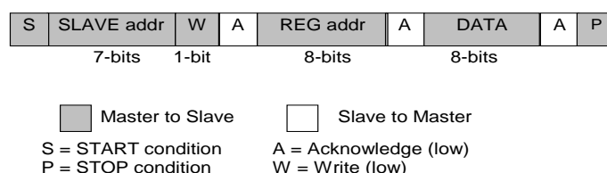
Figure 27: I 2 C Byte Write (SDA signal)
