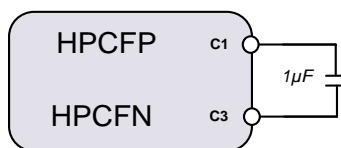
Figure 41: Charge Pump Flying Capacitor
