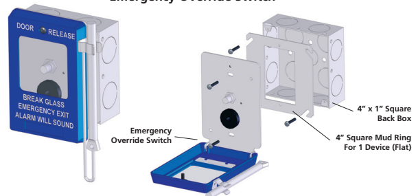
Typical Installation of an Emergency Override Switch
