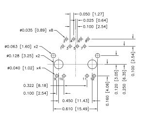
Recommended PCB Layout (Component Side)
