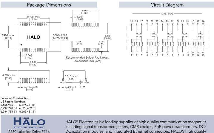
including signal transformers, filters, CMR chokes, PoE power transformers, DC/ DC isolation modules, and integrated Ethernet connectors. HALO's high quality and competitively priced leading edge technology solutions are manufactured in ISO9001 and ISO14001 factories.
