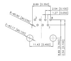
Recommended PCB Layout (Top View)
