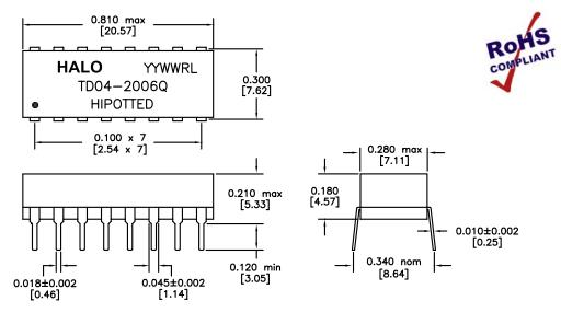
DIMENSIONS: Inch [mm] TOLERANCES: ±0.005 INCH IF NOT SPECIFIED
