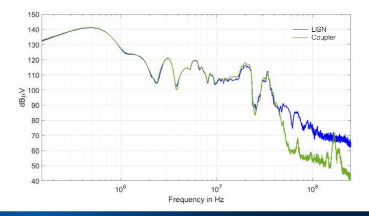
The newly developed HPK Measurement Coupler from Rosenberger enables a minimally invasive testing method in order to measure reliable RF voltages and currents.
