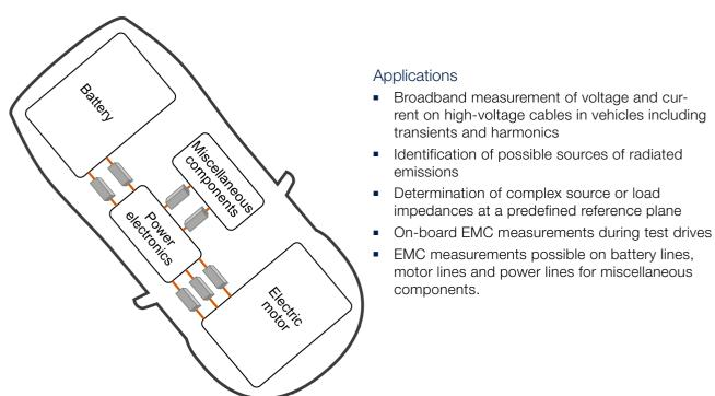
Schematic drawing of a vehicle's traction network including potential positions of couplers
