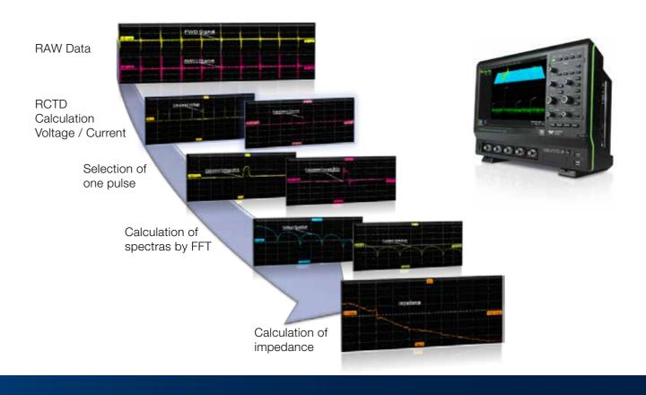
As an additional feature, the post-processing algorithms have been adapted to run on LeCroy HDO oscilloscopes equipped with the XDEV option to allow real-time evaluation of the measurement results.
