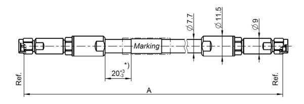
All dimensions are in mm; tolerances:  $\pm$  3mm for A  $\leq$  300 mm;  $\pm$  1% for A > 300 mm \*) If length "A" < 150 mm marking is mount centric  $\pm$ 5 mm
