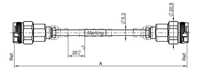
All dimensions are in mm; tolerances:  $\pm$  3mm for A  $\leq$  300 mm;  $\pm$  1% for A > 300 mm \*) If length "A" < 150 mm marking is mount centric  $\pm$ 5 mm
