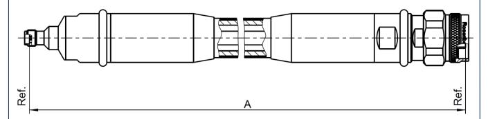
All dimensions are in mm; tolerances: ± 3mm for A ≤ 300 mm; ± 1% for A > 300 mm
