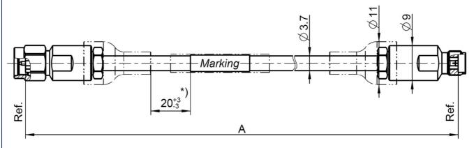
All dimensions are in mm; tolerances:  $\pm$  3mm for A  $\leq$  300 mm;  $\pm$  1% for A > 300 mm\*) If length "A" < 150 mm marking is mount centric  $\pm$ 5 mm
