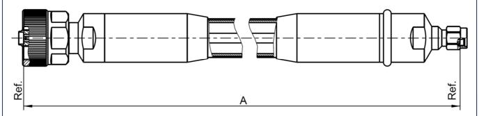
All dimensions are in mm; tolerances:  $\pm$  3mm for A  $\leq$  300 mm;  $\pm$  1% for A > 300 mm
