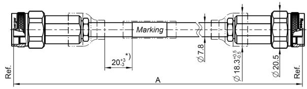
All dimensions are in mm; tolerances: ± 3mm for A ≤ 300 mm; ± 1% for A > 300 mm
