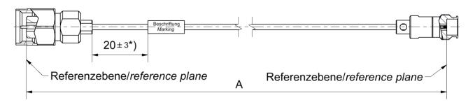
All dimensions are in mm; tolerances: ± 3mm for A ≤ 300 mm; ± 1% for A > 300 mm \*) If length "A" ≤ 90 mm marking is mount centric ± 5mm
