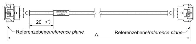
All dimensions are in mm; tolerances:  $\pm$  3mm for A  $\leq$  300 mm;  $\pm$  1% for A > 300 mm \*) If length "A"  $\leq$  90 mm marking is mount centric  $\pm$  5mm
