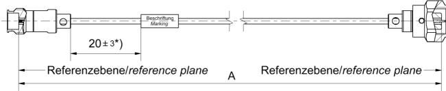
All dimensions are in mm; tolerances:  $\pm$  3mm for A  $\leq$  300 mm;  $\pm$  1% for A > 300 mm
