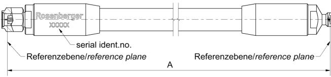
All dimensions are in mm; tolerances: ± 3mm for A ≤ 300 mm; ± 1% for A > 300 mm
