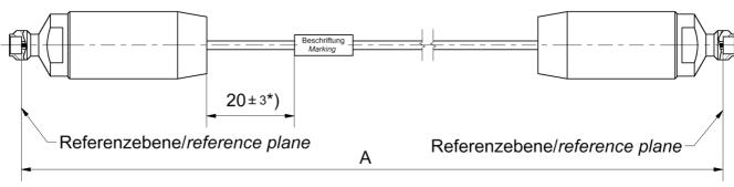
All dimensions are in mm; tolerances:  $\pm$  3mm for A  $\leq$  300 mm;  $\pm$  1% for A > 300 mm \*) If length "A"  $\leq$  90 mm marking is mount centric  $\pm$  5mm
