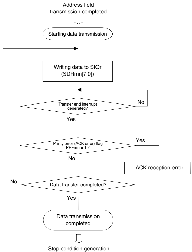
Figure 14-104. Flowchart of Data Transmission
