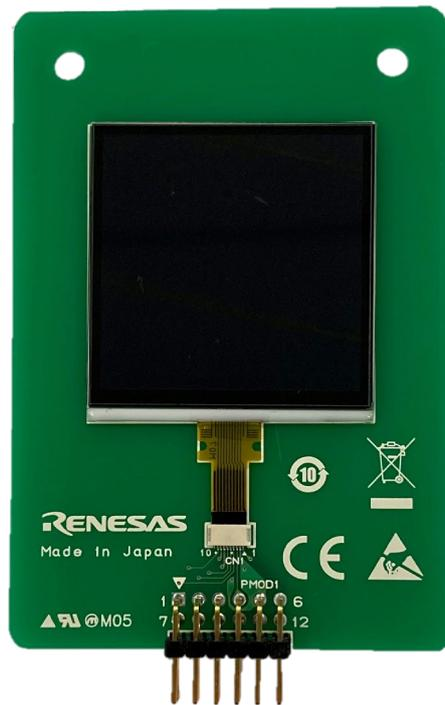
Figure 1-3: MIP-LCD Expansion Board (Top)
