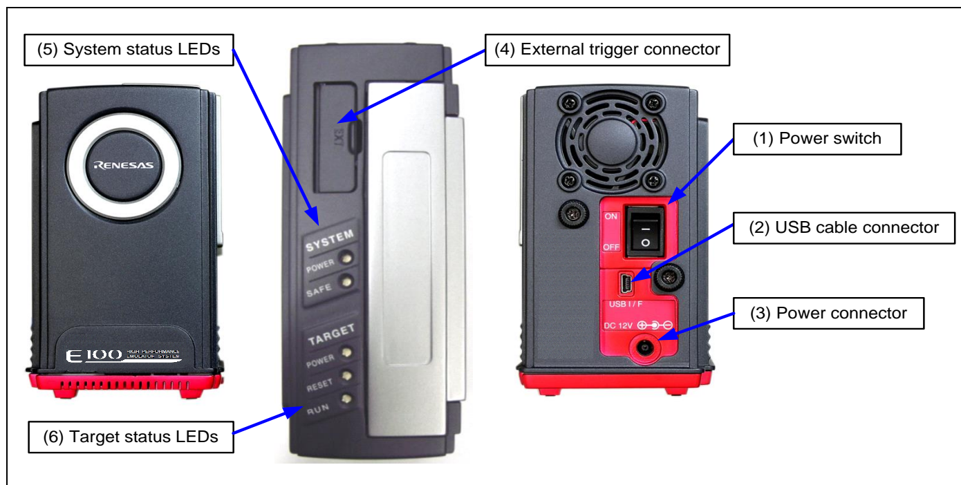
Figure 1.2 Names of the emulator parts
