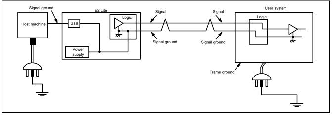
Figure 2.5 Connecting System Ground
