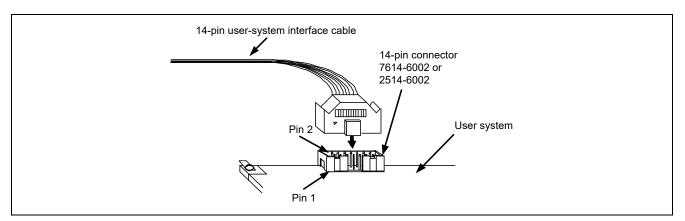
Figure 2.3 Connecting the User-System Interface Cable to the 14-Pin Connector when the E2 Lite is to be Used
