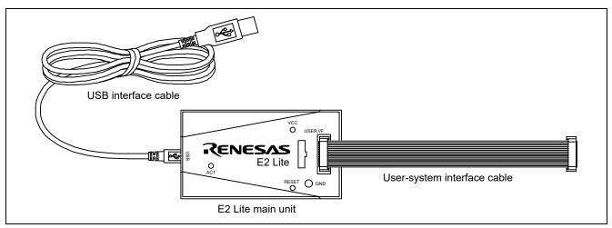
Figure 1.2 E2 Lite Hardware Configuration
