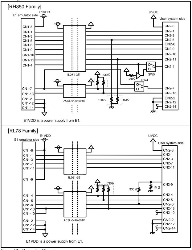
Figure 4.2 Connection Diagrams
