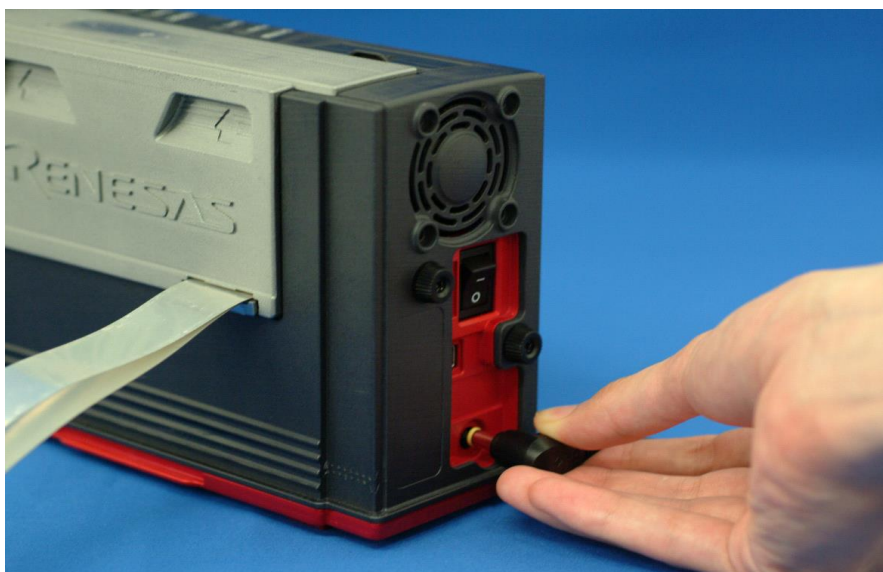
Figure 2.5 Connecting the emulator power supply
