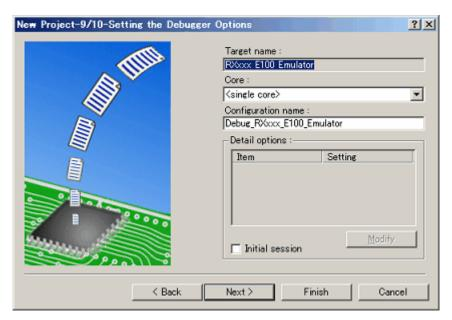
Figure 4.9 [Setting the Debugger Options] Dialog Box
