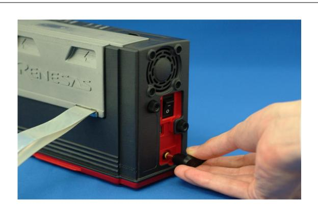
Figure 2.5 Connecting the Emulator Power Supply
