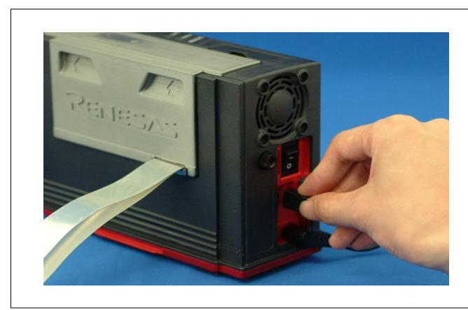
Figure 2.4 Connecting the Host Machine
