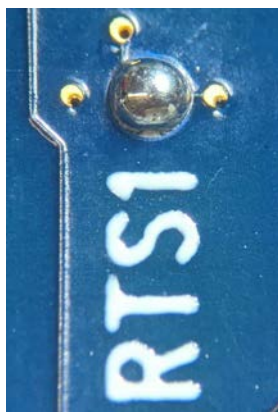
Figure 39. Single Soldering Iron on Solder Bridge
