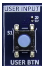
Figure 16. User Switch (S1) on the Target Board
