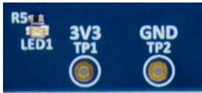
Figure 7. TP1, TP2, and LED1 on the Target Board
