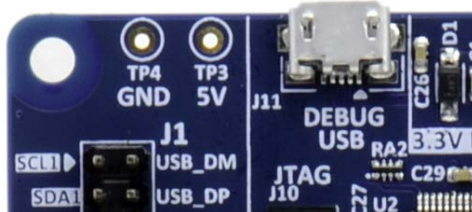
Figure 6. USB Debug Connector (J11), TP3, and TP4 on the Target Board
