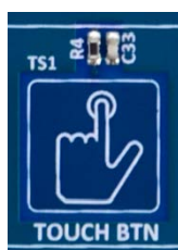
Figure 21. Capacitive Touch Button on the Target Board (Top side)
