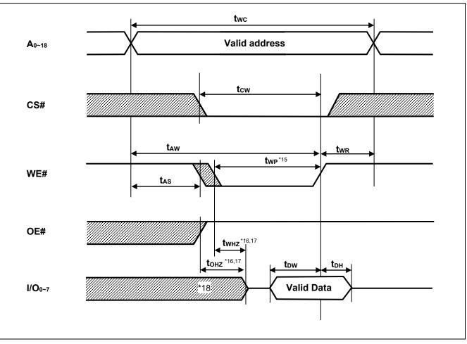
Note 15. twp is the interval between write start and write end. A write starts when both of CS# and WE# become active. A write is performed during the overlap of a low CS# and a low WE#. A write ends when any of CS# or WE# becomes inactive.
