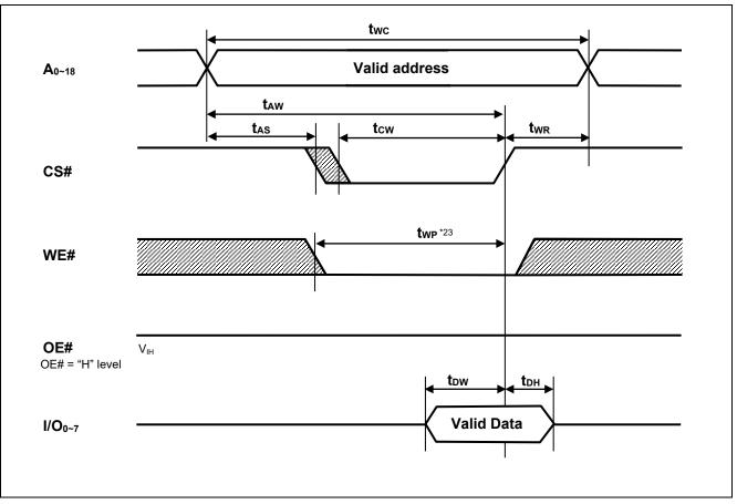
Note 23.  $t_{WP}$  is the interval between write start and write end.
