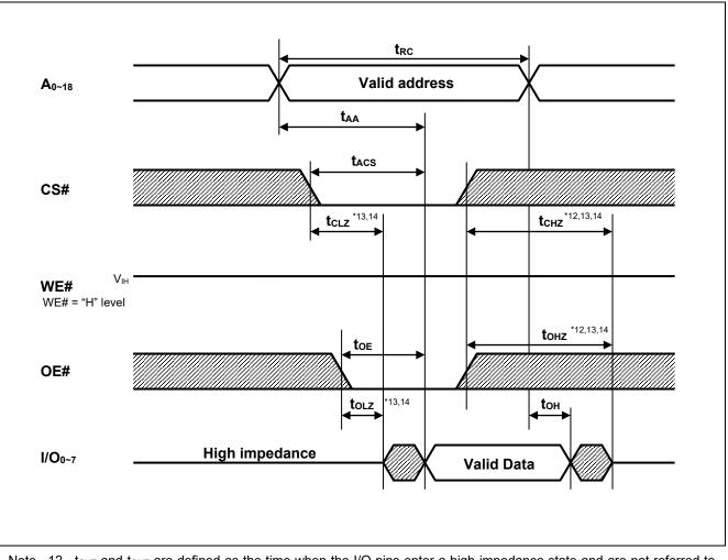
Note 12. t<sub>CHZ</sub> and t<sub>OHZ</sub> are defined as the time when the I/O pins enter a high-impedance state and are not referred to the I/O levels.
