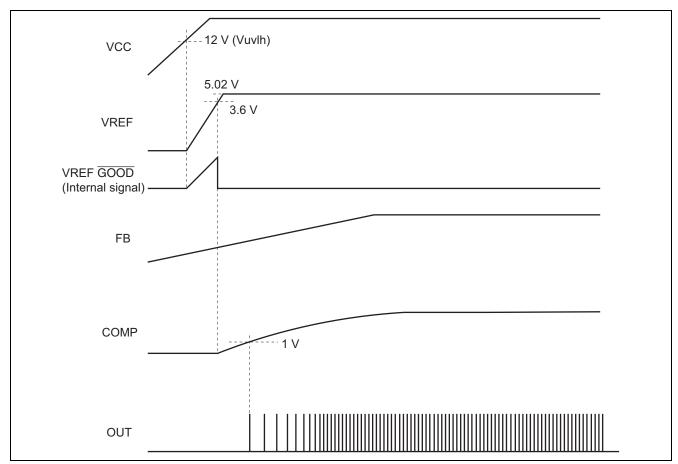
1. Start-up Timing (Zero Current Detection Mode/Fixed Frequency Mode common)
