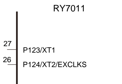
Figure 6 – 5 Connection of the XT1 and XT2/EXCLKS Pins When an On-Chip Oscillator Is in Use Note
