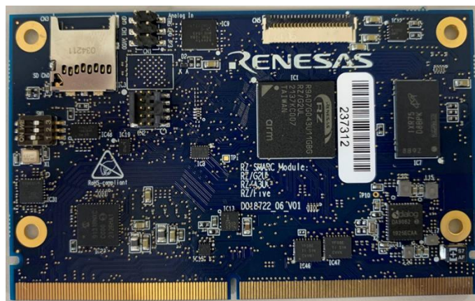
Figure 5.1 Top View of the SMARC Module Board
