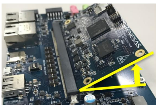
Figure 4.6 How to remove the SMARC Module Board
