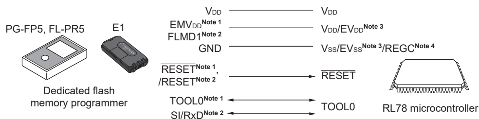
Figure 33-2. Communication with Dedicated Flash Memory Programmer
