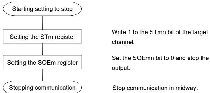
Figure 15-123. Procedure for Stopping UART Transmission
