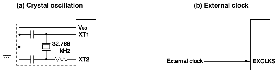
Figure 5-24. Example of External Circuit of XT1 Oscillator
