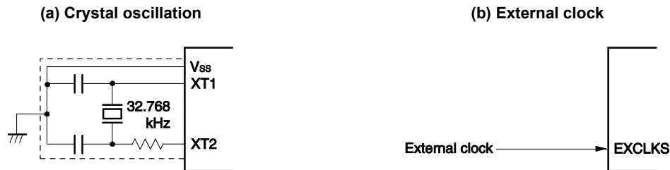
Figure 5-24. Example of External Circuit of XT1 Oscillator
