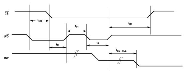
FIGURE 2. SERIAL INTERFACE TIMING DIAGRAM DECREMENT
