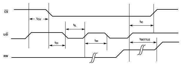
FIGURE 1. SERIAL INTERFACE TIMING DIAGRAM, INCREMENT
