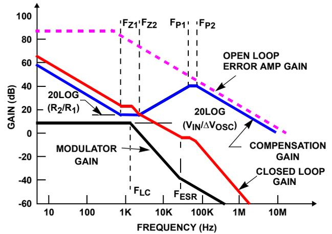
FIGURE 4. ASYMPTOTIC BODE PLOT OF CONVERTER GAIN
