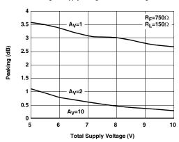
Peaking vs Supply Voltage for Inverting Gains
