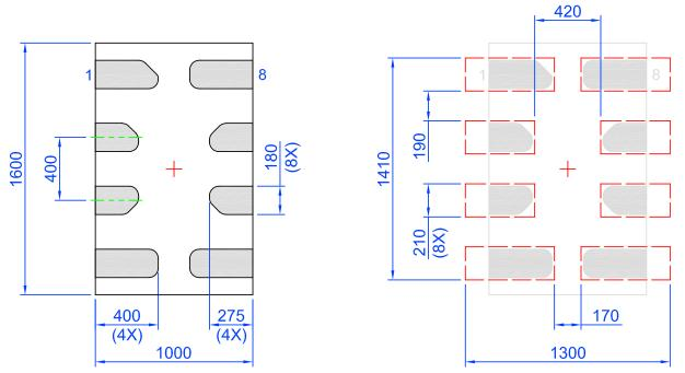
Note: All dimensions shown in micrometers (μm)
