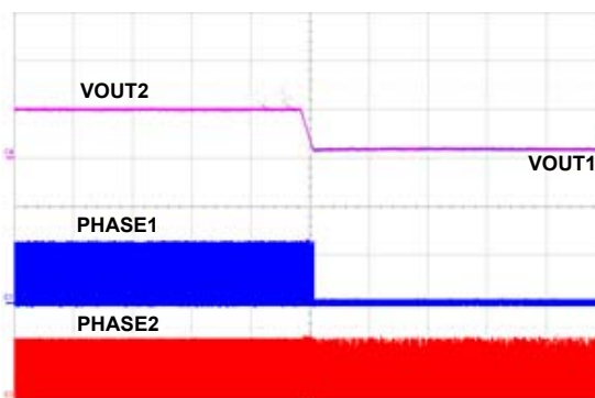
Figure 6. VOUT2 Tracking VOUT1 when Channel 1 is Disabled
