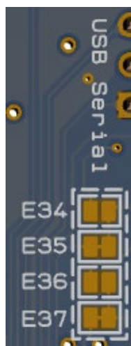
Figure 24. USB to Serial Copper jumpers (bottom side)
