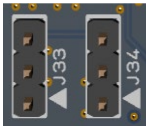
Figure 18. Pmod 2 Pin header jumpers (top side)
