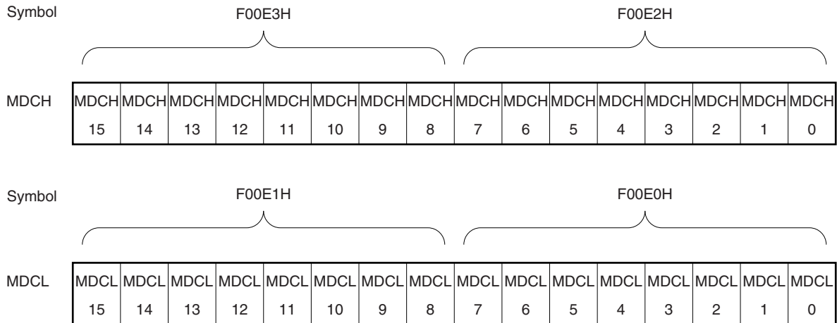
Figure 15-4. Format of Multiplication/Division Data Register C (MDCH, MDCL)
