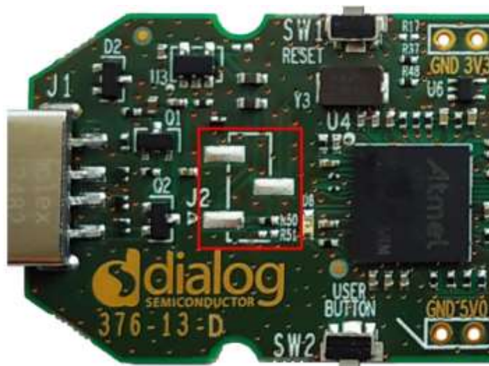
Figure 25: Current Measurement Header (J2)
