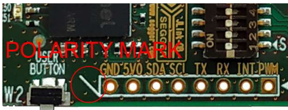
Figure 18: Guides for Proper MikroBus™ Click Board Insertion
