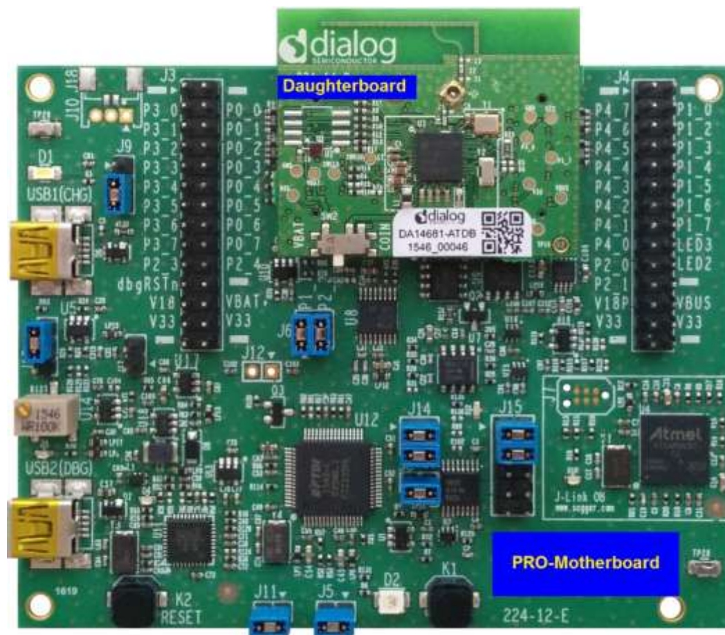
Figure 1: PRO development kit, motherboard and daughterboard
