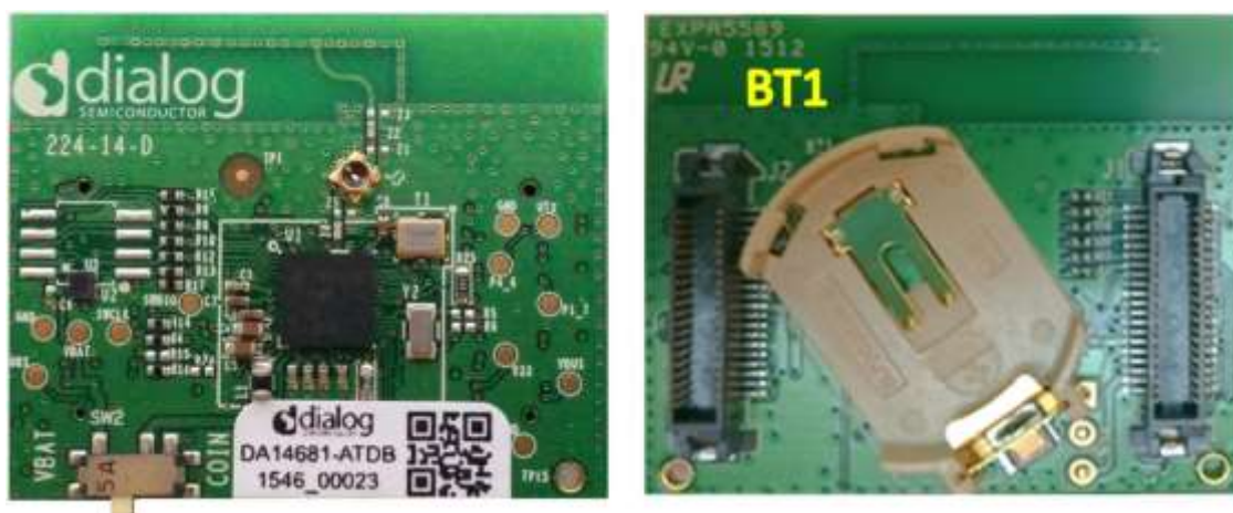
Figure 34: DA1468x/DA1510x daughterboard power source selection
