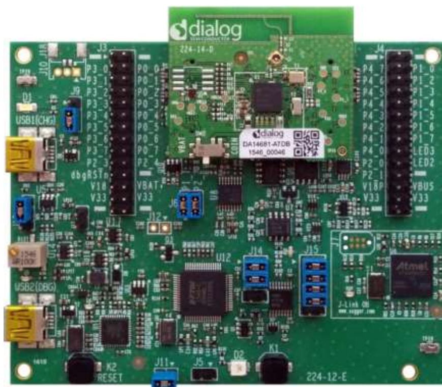
Figure 13: Jumper's placement for Full UART functionality
