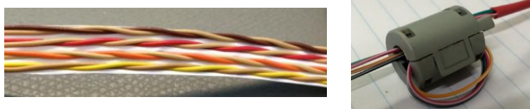
Figure 164: Example of Twisted Pair Cable with 4 Pairs and Ferrite
