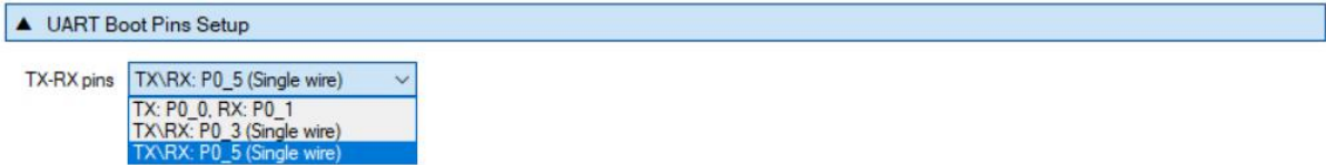
Figure 45: UART Boot Pins Setup - DA14531
