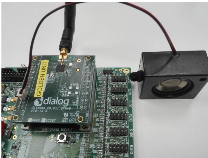
Figure 169: Speaker Connection for Audio Test.
