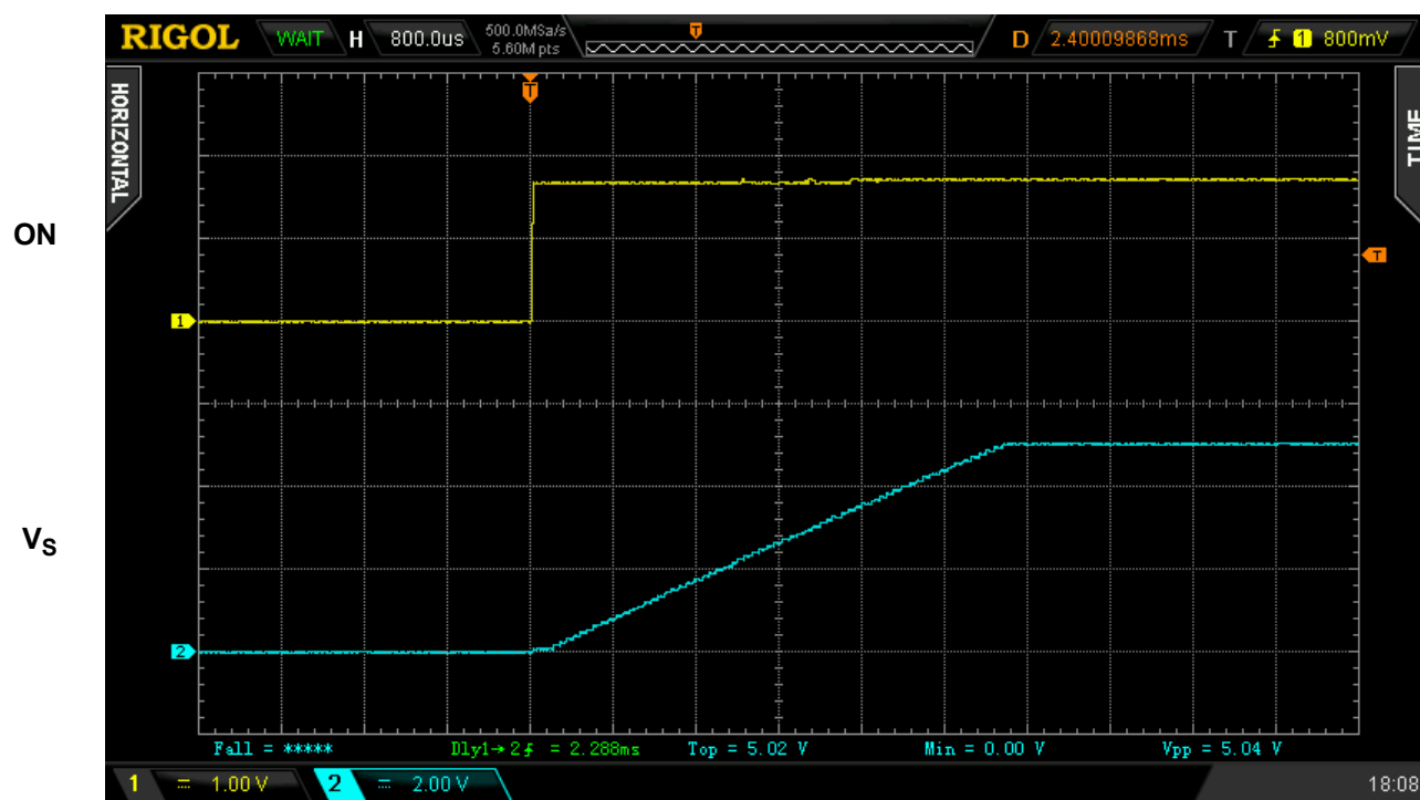
Figure 2. Typical Turn ON operation waveform for V_{DD} = V_D = 5\text{ V} , C_{SLEW} = 12\text{ nF} , C_{LOAD} = 10\text{ }\mu\text{F} , R_{LOAD} = 20\text{ }\Omega
