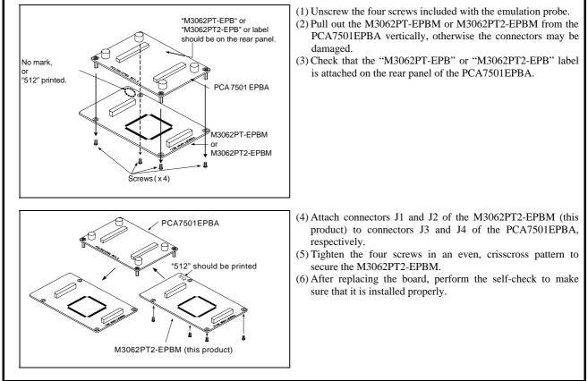
Figure 3.1 Replacing the MCU board
